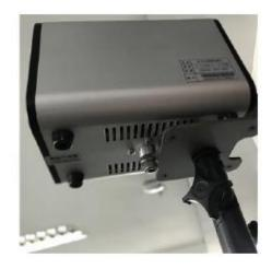
**Note:** Once the blackbody is installed, raise the tripod to 6ft (1.8m) and in sight of the camera's lens. Plug the blackbody into a power source such as a surge protector or wall outlet and allow the device to preheat for 30 minutes before use. Be sure not to run the cable in areas of high traffic or where they can be trampled on or damaged.
